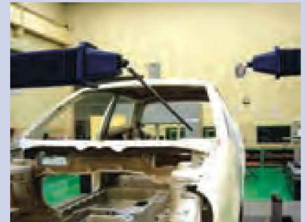
Measurement example for dual type (Equipped with touch-trigger probe and line laser probe)
