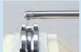
Inner/outer ring contour of a bearing
