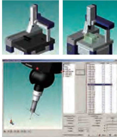
Example of sampling method: touch measurement
