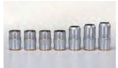
BD (Bright / Dark field) for observation/measurement
