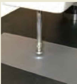
Thickness measurement of non-metallic sheet
