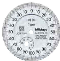
Graduation: 0.001mm, Measuring range: 1mm 1109S-10 Shockproof Jeweled bearing
