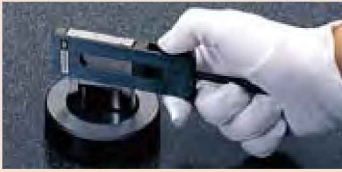
Gaging a bore using a pair of half round jaws and a holder
