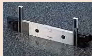
Use of B-type connectors in gage construction
