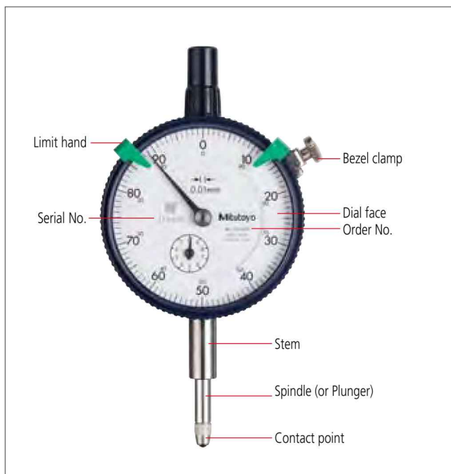
Parts of a dial indicator
