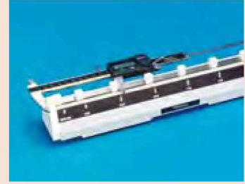
Checking accuracy of caliper (outside measurement)
