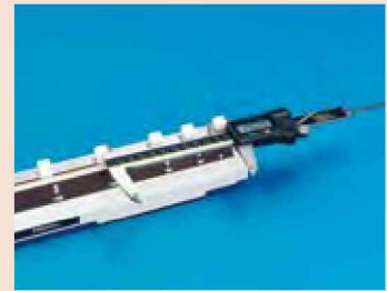
Checking accuracy of caliper (inside measurement)
